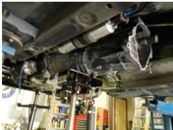
Figure 2 Success! Tranny remounted
